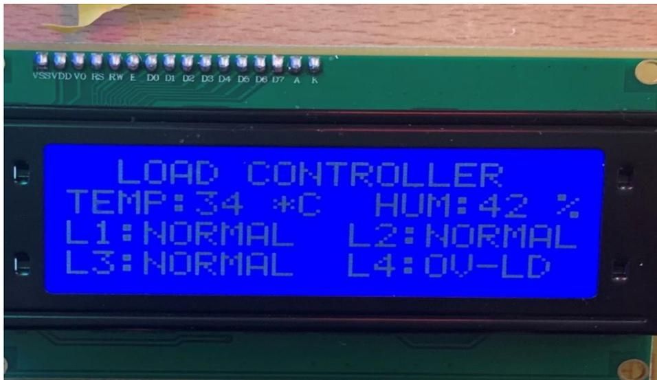
**Figure 4.3 when circuit has overload circuit**
