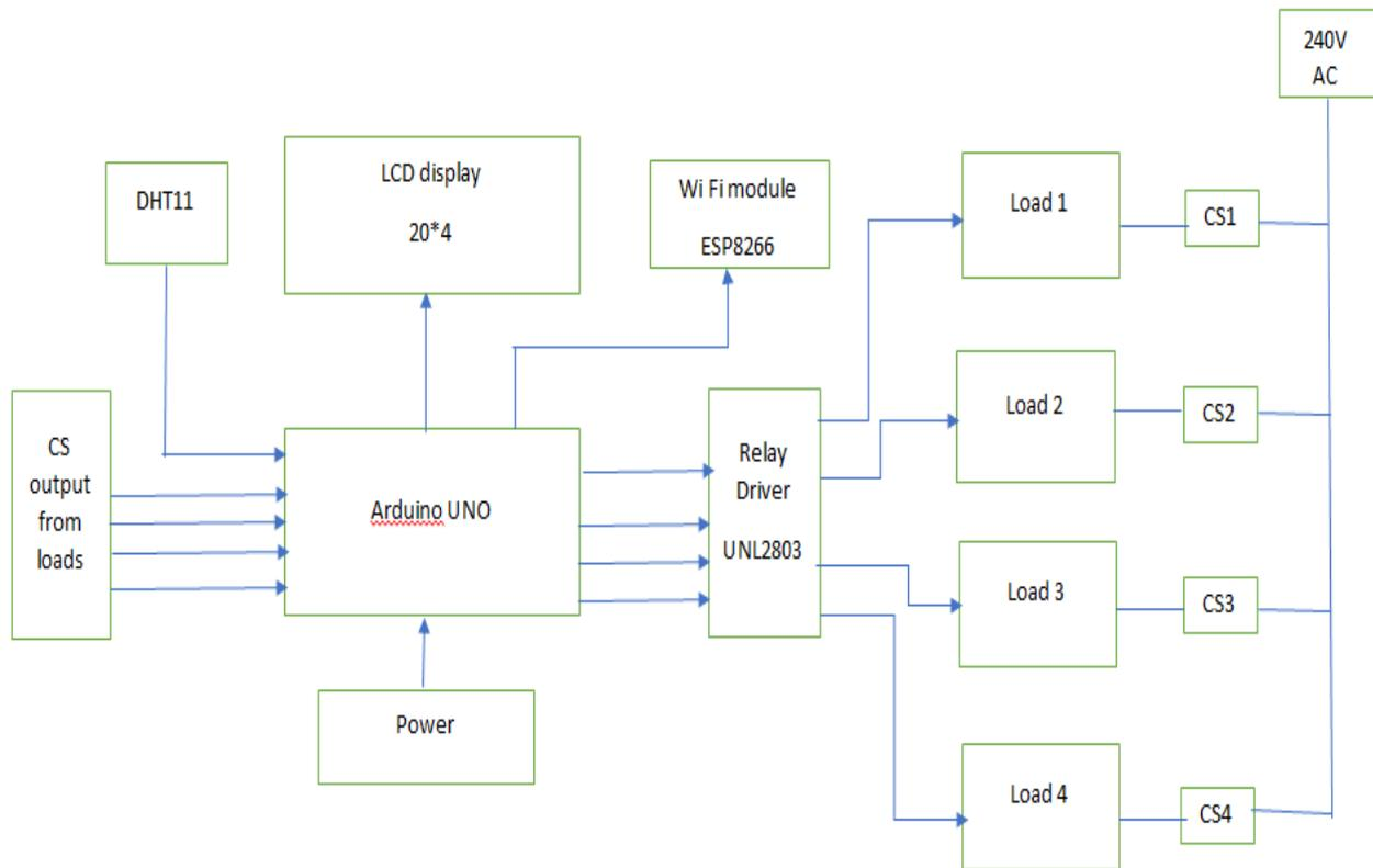
**Figure 3.1 Block Diagram**
