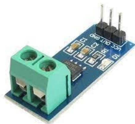
**Figure 2.5 Current Sensor<sup>5</sup>**
