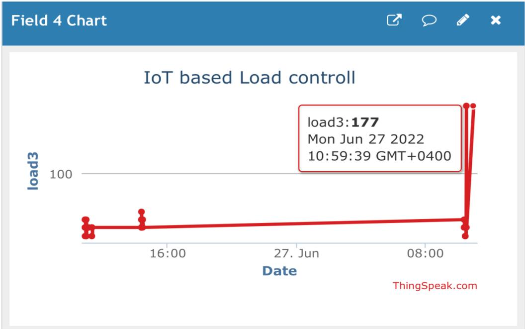
Figure 4.9 Load3 graph when occur short circuit
