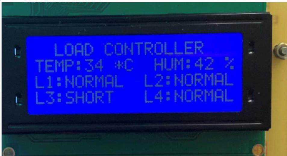
Figure 4.2 when circuit has short circuit
