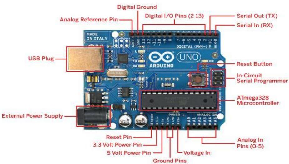
**Figure 2.1 Schematic Diagram of Arduino <sup>1</sup>**
